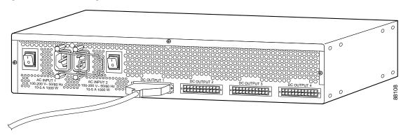
Figure 15 Connecting a Two-to-One Y-Cable to a Cisco RPS for Fully Redundant Power
